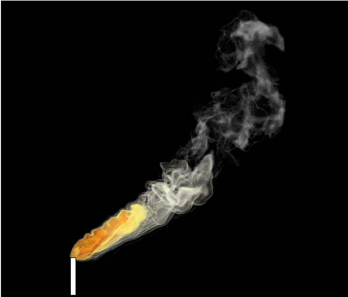
Figure 3: Predicted Flame Shape for 10 inch Diameter Well Test Flare
