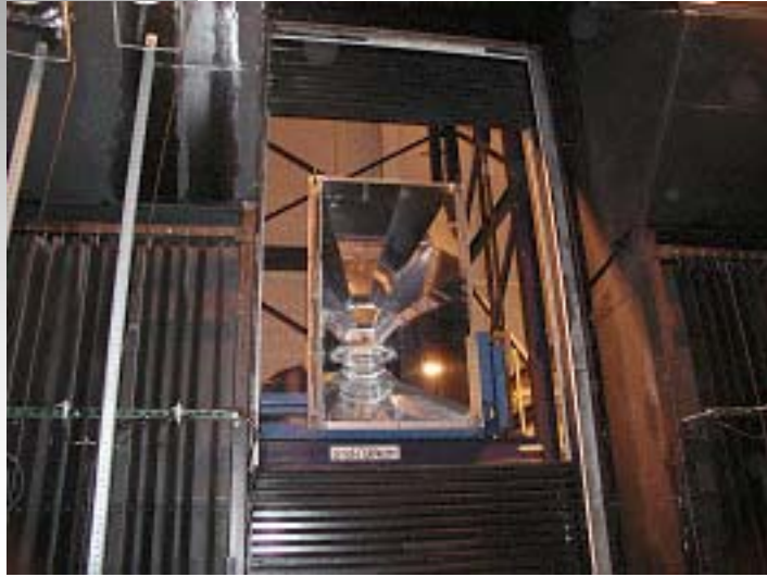
National Solar Testing Facility (NSTF) 150 kW Vortek solar simulator (150-1120 watts per square meter)
