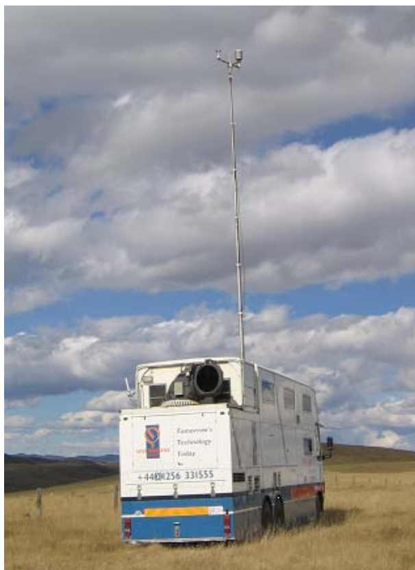
Figure 1: Rear of DIAL Mobile Unit Showing Telescope System
