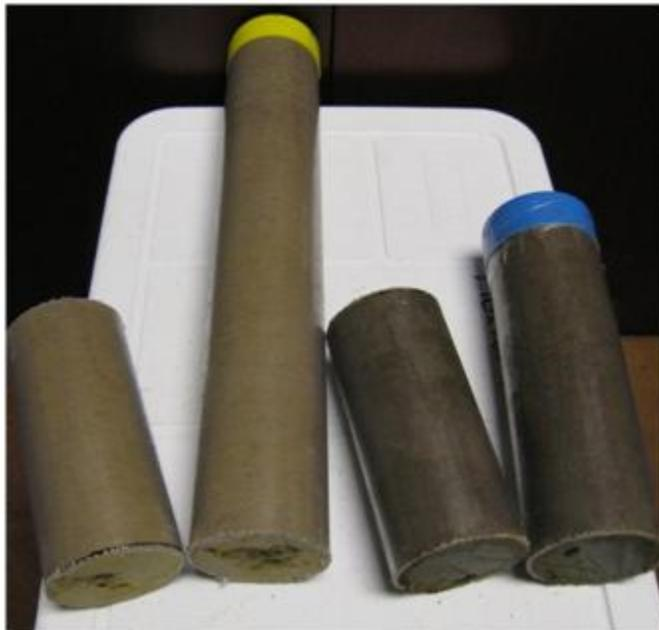
Samples without apparent channels could be tested as ‘undisturbed’ cores in customized shelby-tube permeameters (leaching columns), with an example of such a configuration shown in Figure 4.2. Other cores with significant voids or channels were emptied, homogenized, dried and ground, and sieved through #10 (2 mm) mesh as shown in Figure 4.3. These soil samples can then be tested as ‘repacked’ samples using one or more layers of soil in clear permeameters such as shown in Figure 4.4.
