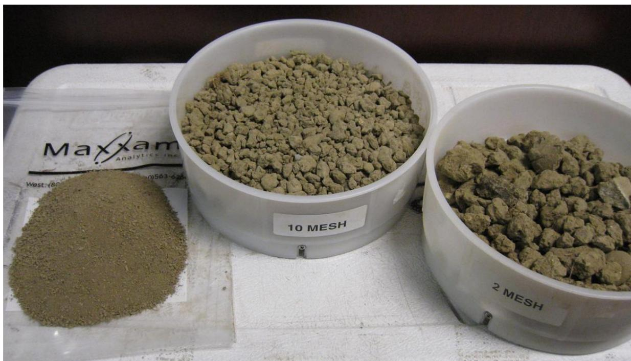
**Figure 4.4. Repacked column with two layers of #10 mesh soil**
